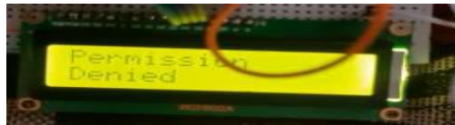
Fig 22. LCD display showing "Permission Denied" message
